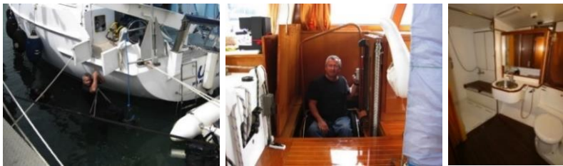
Figure 27. URI's Lift Systems and Bathroom (Wheelchair Sailing, n.d.)
